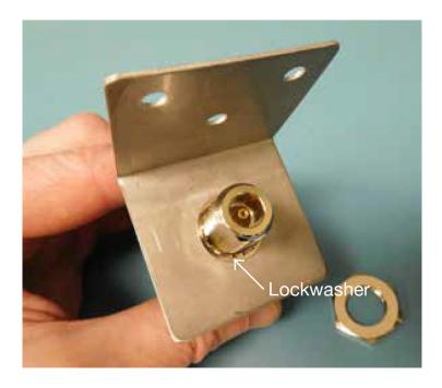
Install the nut and tighten securely with a 1-inch wrench.
