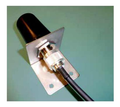
**Step 5** – Insert the cable gland on the SMA end of the cable.
