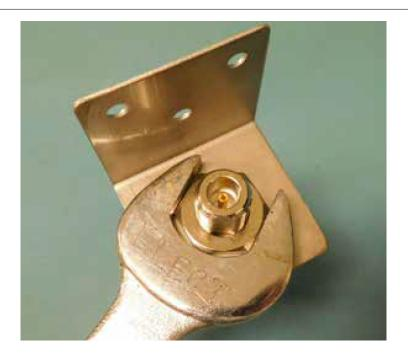
**Step 4** – Connect the coaxial cable to the antenna with the N-connector.
