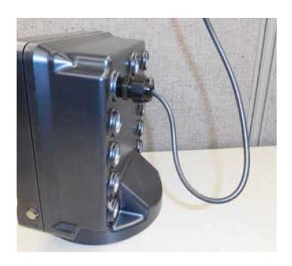
**Step 11** – Attach the cable securely to the vehicle using wire ties or insulated wire clamps. The cable requires no special standoffs.
